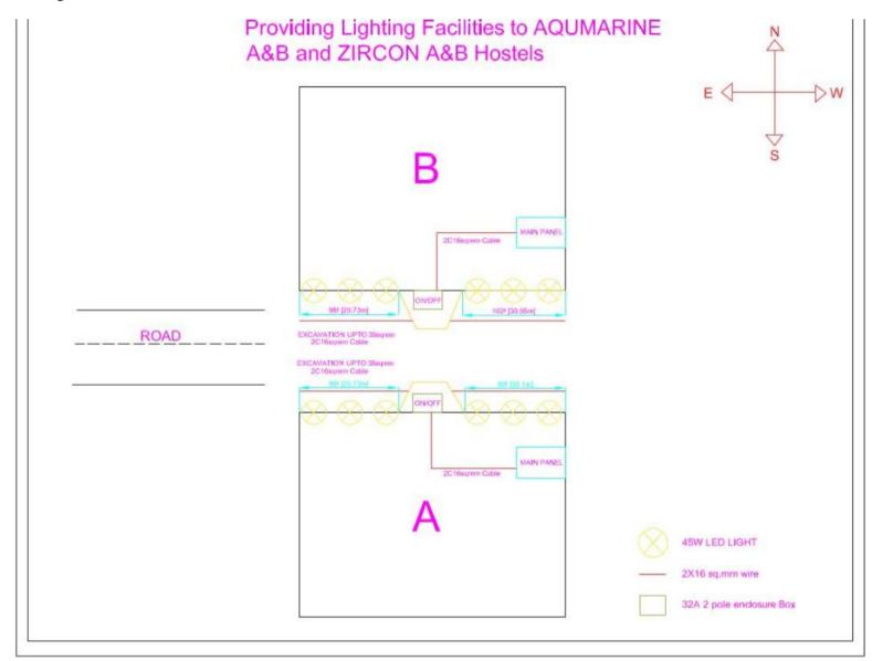
4 sq.mm wire with 20mm PVC 32A 2 pole enclosure Box
